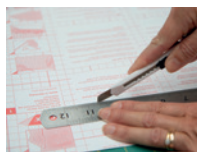
2. Cut the film to size using the backing paper.
